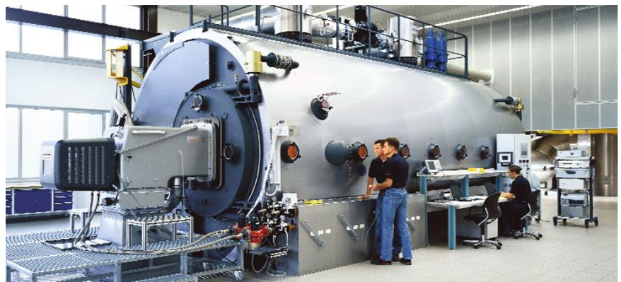
*Burners rated up to 32 MW are tested on the world's largest test firing chamber in the R&D Centre*
