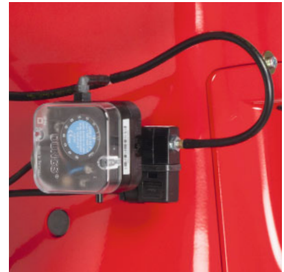
An additional solenoid valve enables the combustion manager to test the air pressure switch, providing a continuously running fan or post purge facility to ensure maximal safety
